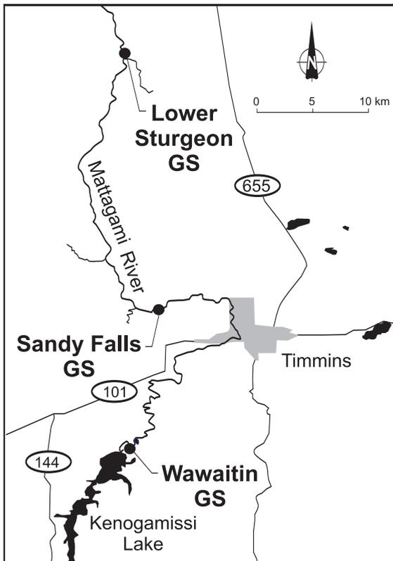
The Proposed Undertaking consists of the following: A new powerhouse will be built at each site. There will also be some refurbishments and modifications made to the existing civil works such as the dams and weirs at each generating station. The existing powerhouses and associated electricity connections will be decommissioned.
