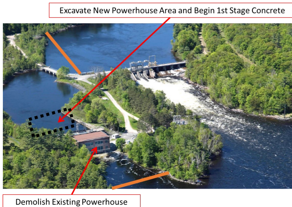
Figure 2-10. Work Sequence – Stage #2 – Powerhouse Demolition and Excavation of New Powerhouse
