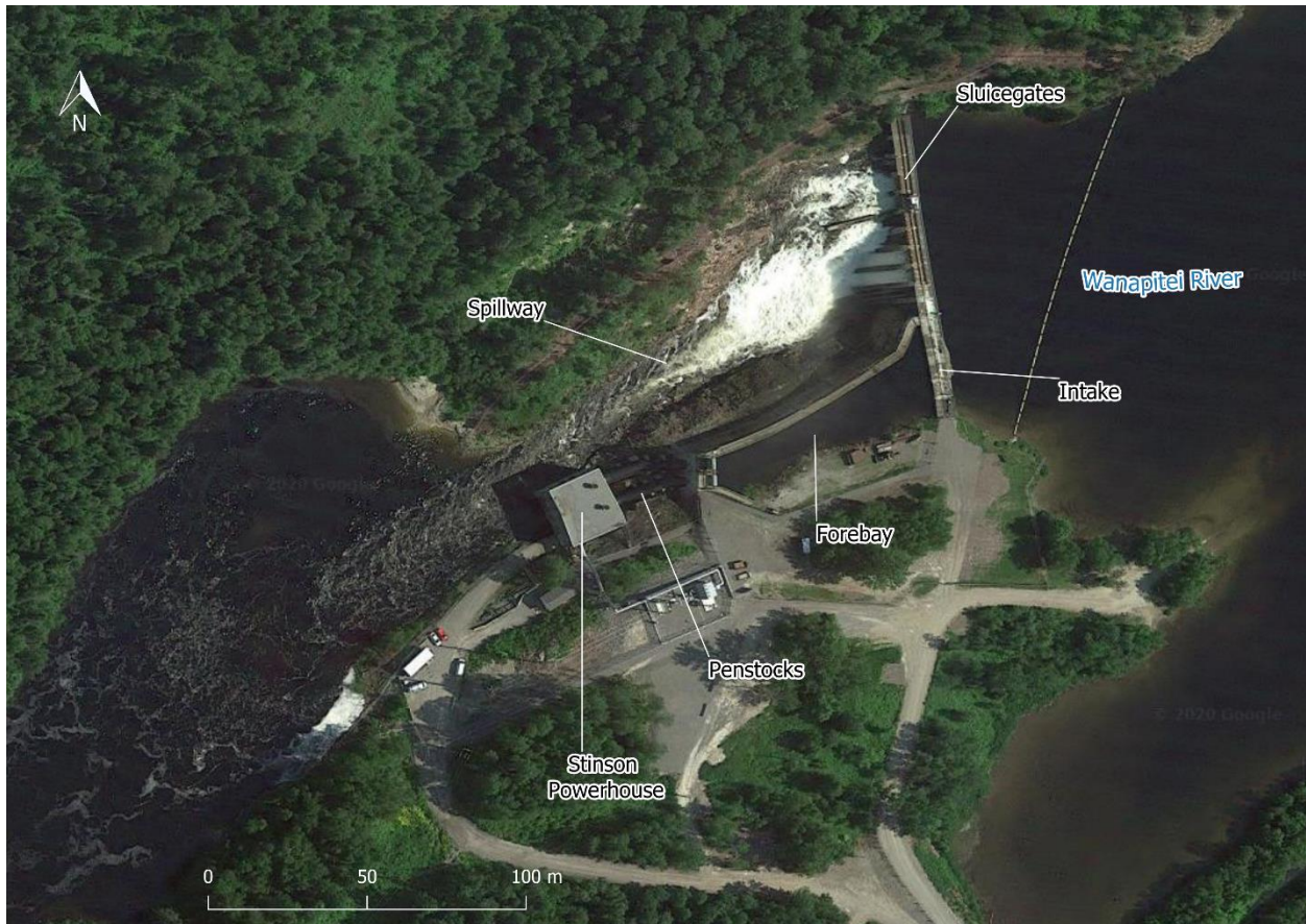
Figure 2-2. Wanapitei River in the vicinity of the Stinson GS. Aerial photo taken on July 2, 2019. Major flow through dam and spillway.
