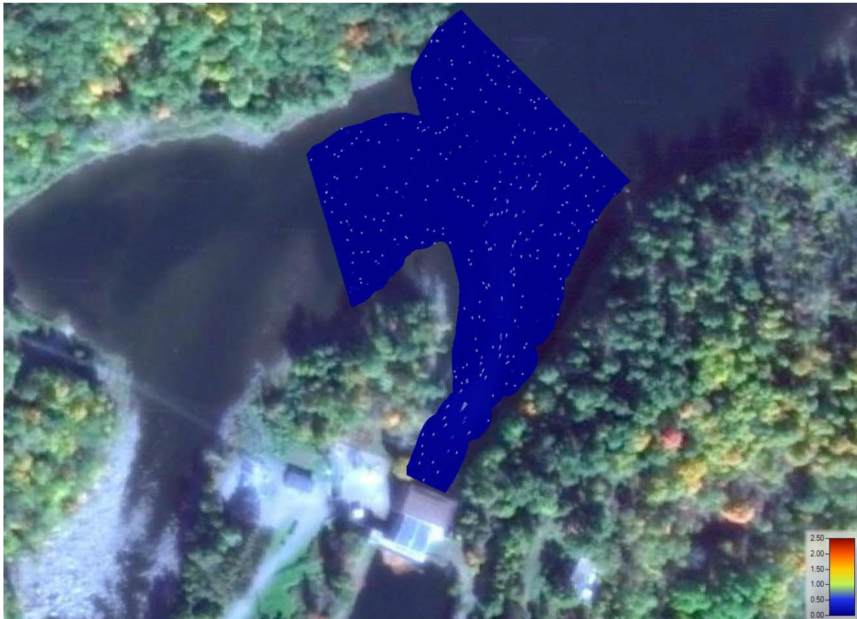
Figure 2-16. Existing Calabogie GS Tailrace Hydraulic Conditions. No Flow
