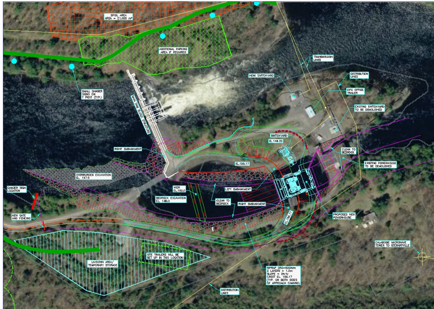
Figure 2-8. Proposed Powerhouse Arrangement for Calabogie
