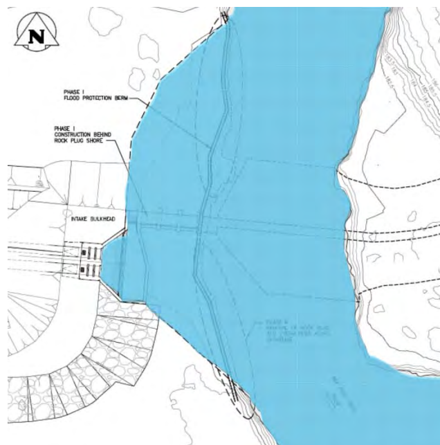
Figure 2.14b Phase II – Removal of Rock Plug
