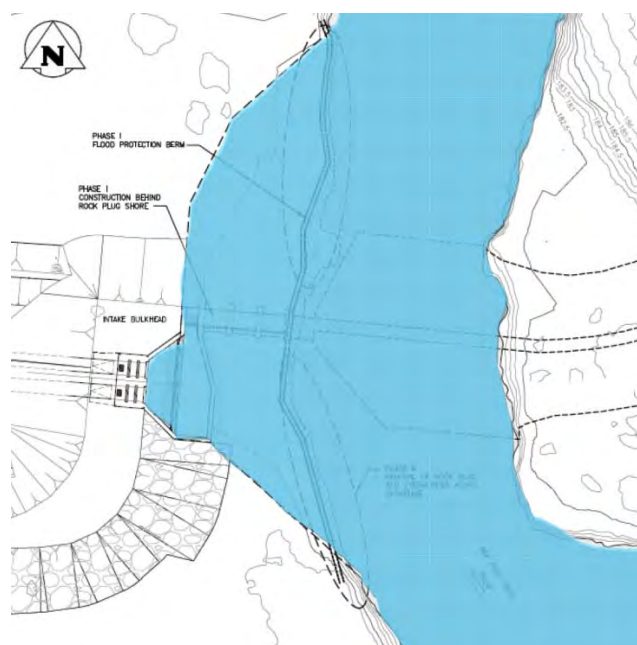
Figure 2.14b Phase II – Removal of Rock Plug
