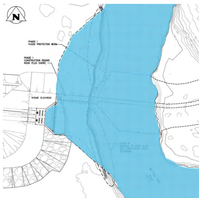
Figure 2.13b Phase II – Removal of Rock Plug
