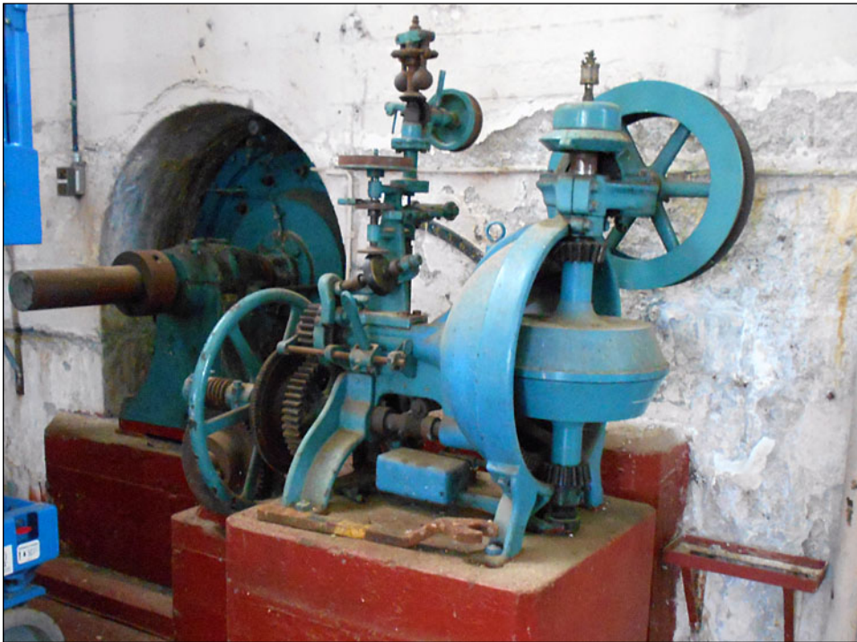
Figure 24. A Woodward governor (right) and turbine (left) at the plant are associated with a former water-driven exciter.
