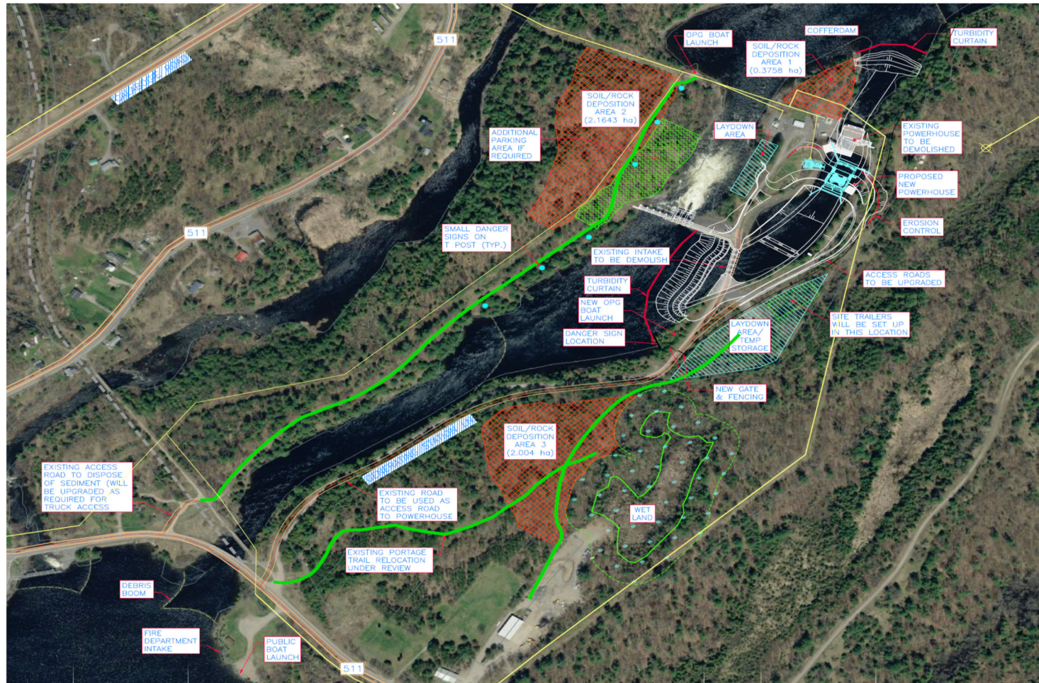
Figure 2-7. Proposed Site Plan for the Calabogie GS
