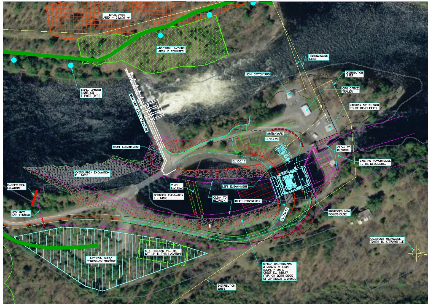
Figure 2-8. Proposed Powerhouse Arrangement for Calabogie
