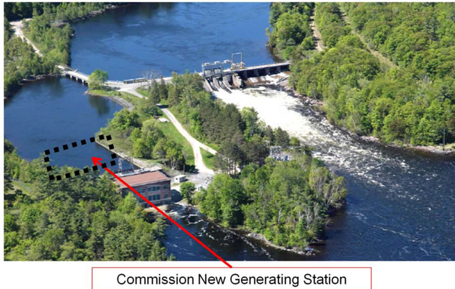
Figure 2-13. Work Sequence – Stage #5 – Commission New Generating Station
