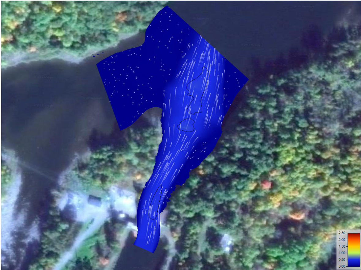
Figure 2-19. Future Calabogie GS Tailrace Hydraulic Conditions. 66 cms Flow (no spill)
