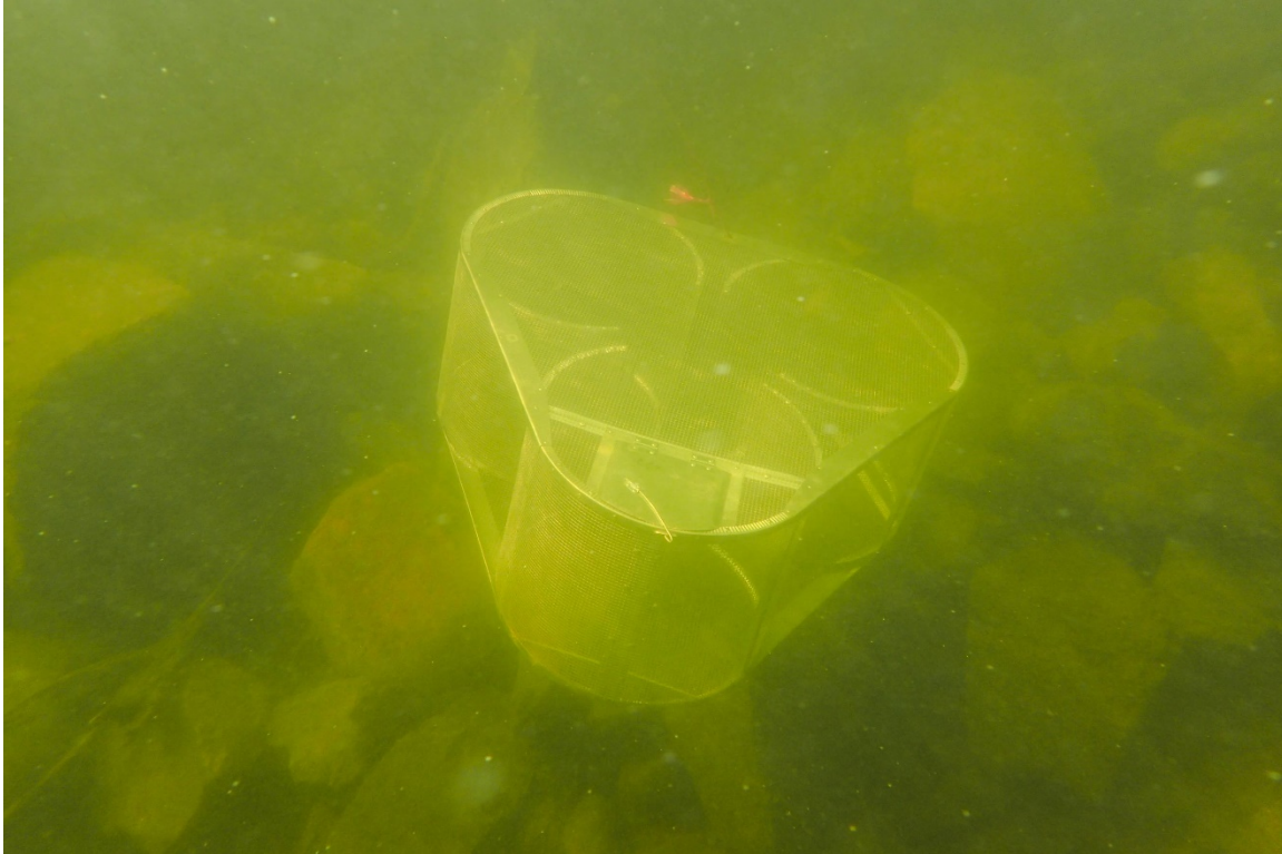
Figure 3-3. Cloverleaf fish trap set on coarse substrate.
