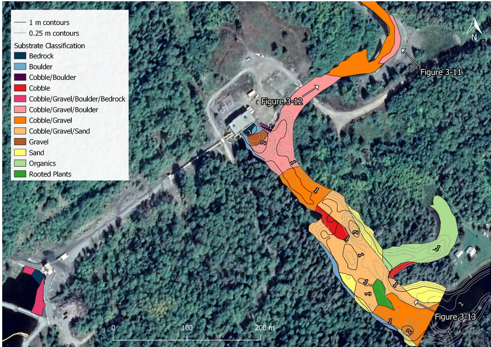
Figure 3-3. Substrate and bathymetry upstream of the intake, within the lower spillway, and immediately downstream of the Matabitchuan GS on July 21-22, 2020. For each substrate class, the size classes are listed in order of decreasing proportion. Location and direction of representative stream habitat photos are also identified using arrows.
